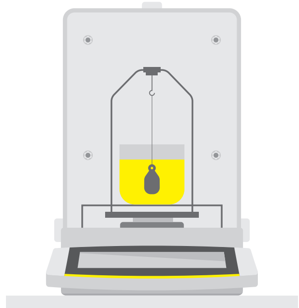
Figure 17: Determination of Liquid Density by the Buoyancy Method
